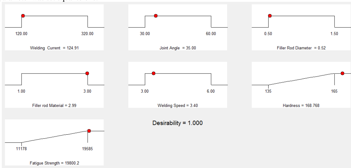
Fig 6: Ramp Function Graph of Desirability for hardness and fatigue strength of welding joint
