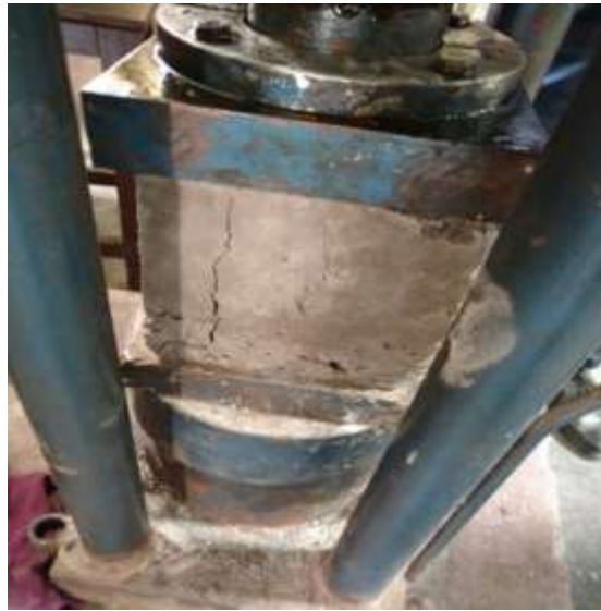
Figure 4: Cube after failure
