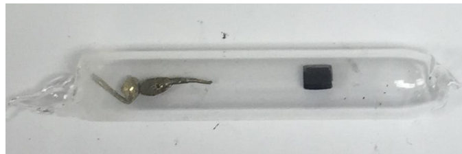
Fig. 1. Sealed quartz ampoule, under a vacuum of 10^{-5} mbar, with two Cd shots and CdMnTe wafer. The length of the ampoule is approximately 5 cm.
