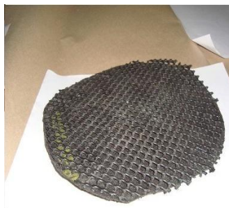
(C) View of Geocomposite(Geotextile + Geogrid)
