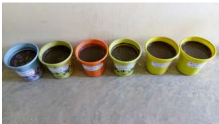
Photo 1.0 Typical pictorial representation of Black Cotton Soil treated (soaked) in Alkaline effluent
