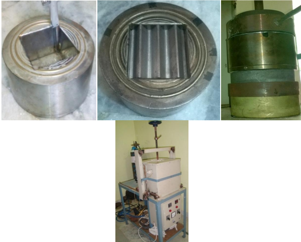
Fig.4 (a) Square die (b) Combination die with square and multi V groove (c) Die assembly (d) Experimental set up
