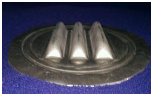
Fig.6. Formed multi V grooved component
