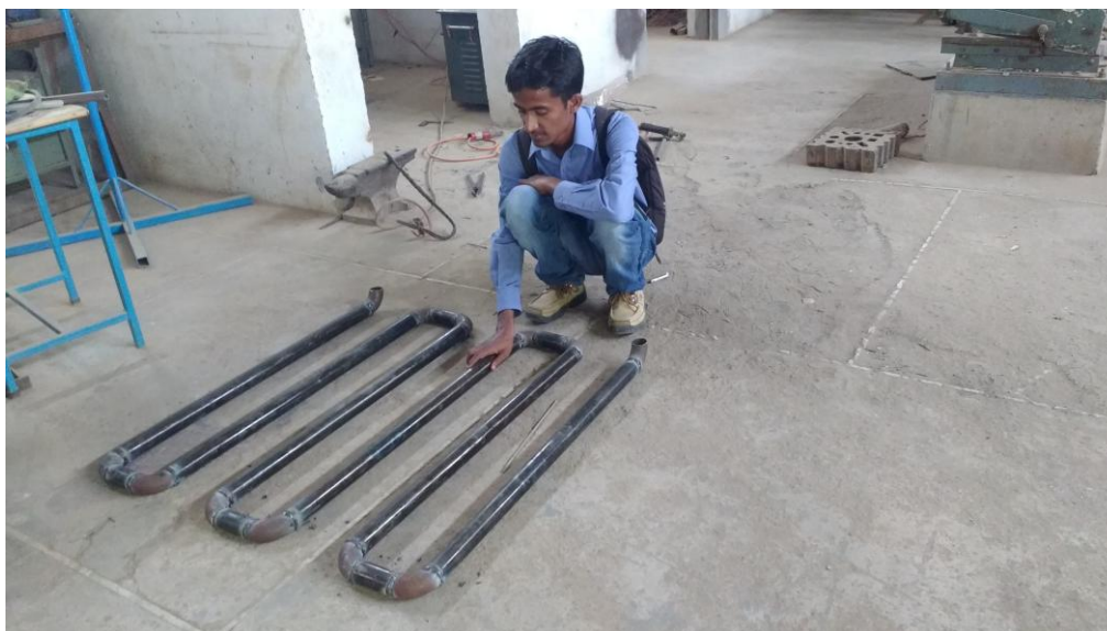
Fig. 4: Series connection of mild steel pipes in mechanical workshop
