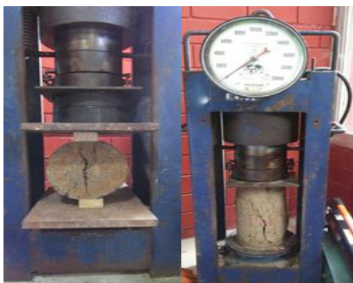
Figure 1.- Crack visualization of specimens with ixtle for: a) tensile test and b) compression test
