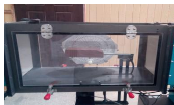
Plate 2: Prototype of Ahmed body (25° slant angle) mounted in the wind-tunnel.
