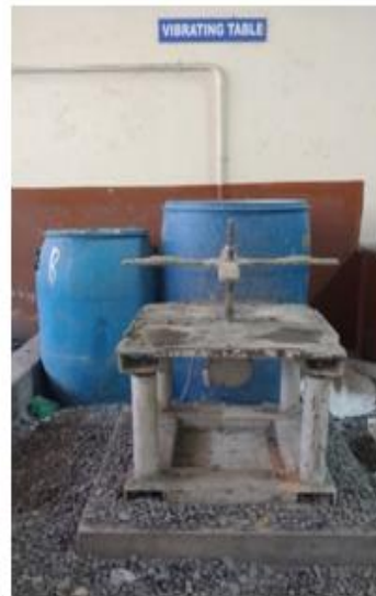
Figure 2 Vibrating Table for compaction of concrete
