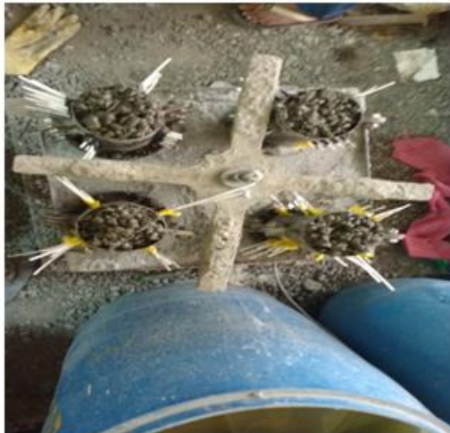
Figure 3 Fibre reinforced cylindrical mould on vibrating table
