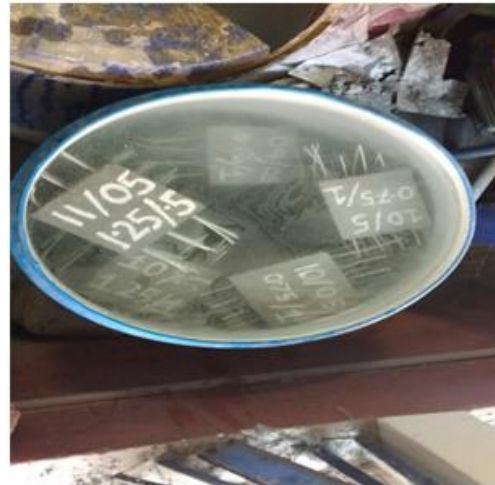
Figure 4 Curing of concrete cubes
