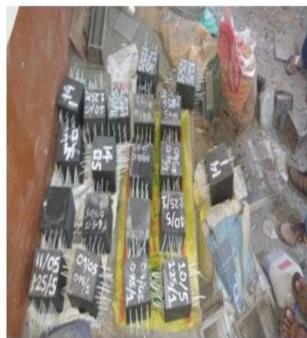
Figure 6 Preparing the concrete cubes for compression test
