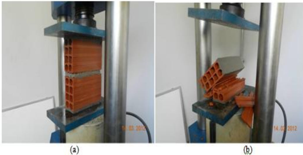
Figure 5. (a) Prism before test,(b) Prism after test
