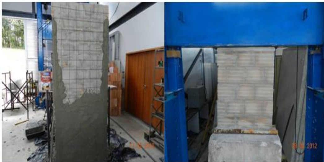
Figure 3. (a) Wall of 1,20 m x 2,60 m with roughcast and plaster, (b) Wall of 0,90 m x 1,04 m with roughcast
