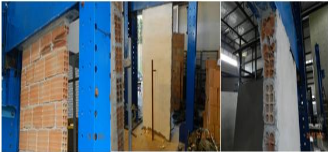
Figure 6. Failure modes of 1,20m x 2,60m walls
