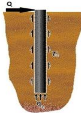
Figure 22 – Pile-soil behaviour upon lateral load
