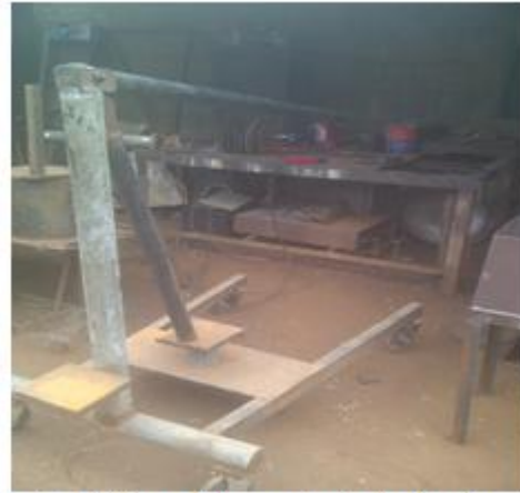
Plate 4. Fitting of the arm to the hydraulic crane assembly
