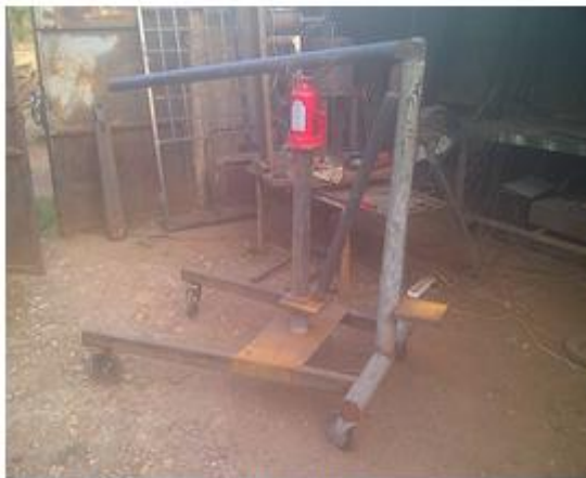
Plate 5. Crane assembly with hydraulic jack fixed
