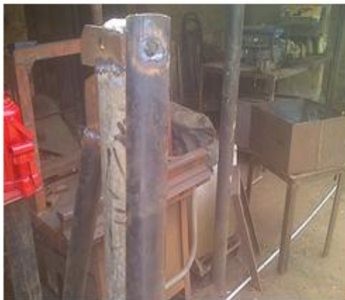
Plate 1. Drilled Hole on one end of the crane's arm
