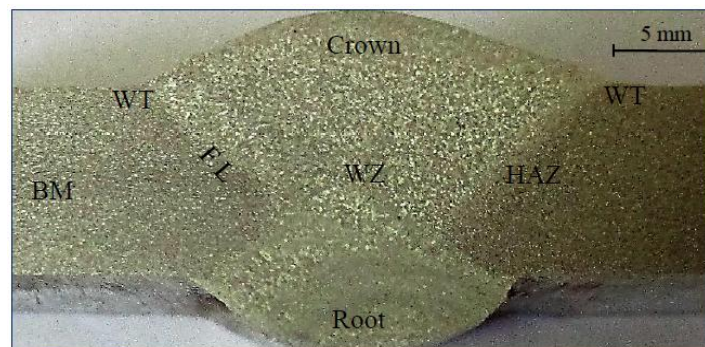
Fig. 8 Cross section analysis of MIG welded AA5083-H111: base metal (BM), fusion line (FL), weld zone (WZ), heat affected zone (HAZ), and weld toe (WT).
