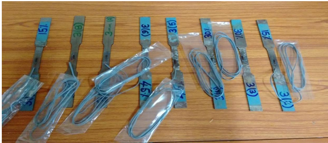
Fig 5: Corroded and uncorroded coupons with strain gauges
