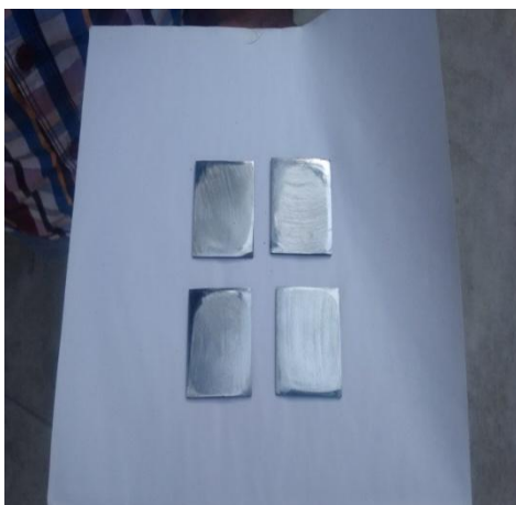
Fig 1: Polished cold formed steel coupons
