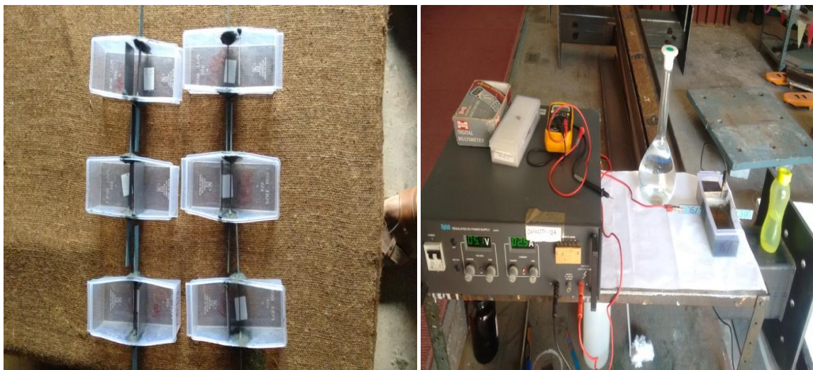
Fig 6: Corrosion – Experimental setup
