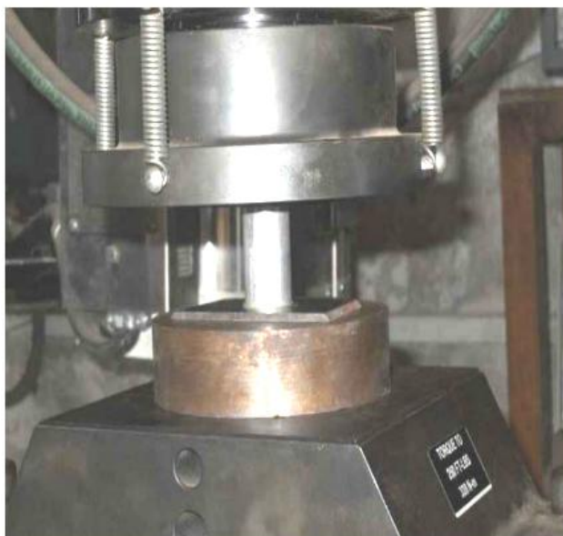
Figure 3.2 Extrusion Die Punch on Universal Testing Machine
