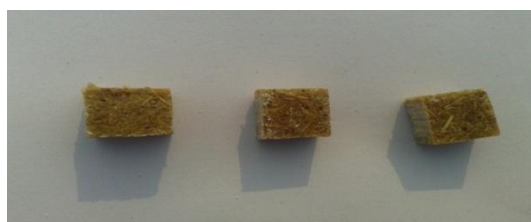
Fig. 6 Hardness test specimens as per ASTM standards
