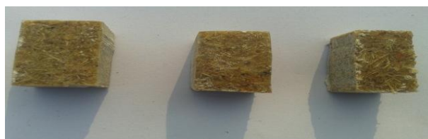
Fig. 3 Tensile Test Specimens as per ASTM standards
