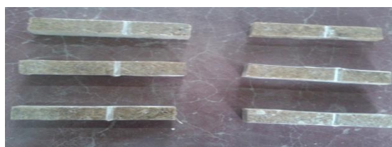
Fig. 5 Impact test specimens as per ASTM standards
