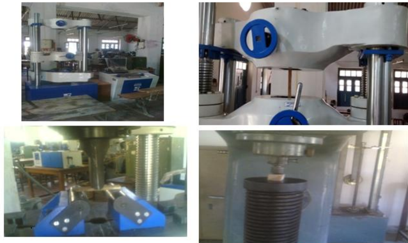
Fig. 7 UTM and other testing set to find mechanical properties of natural composites
