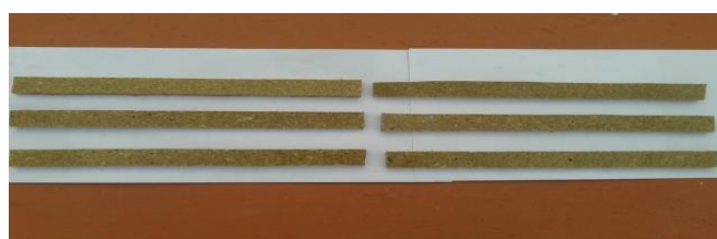
Fig. 4 Flexural test specimens as per ASTM standards
