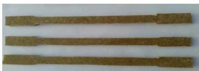
Fig. 2 Tensile Test Specimens Prepared by ASTM standards
