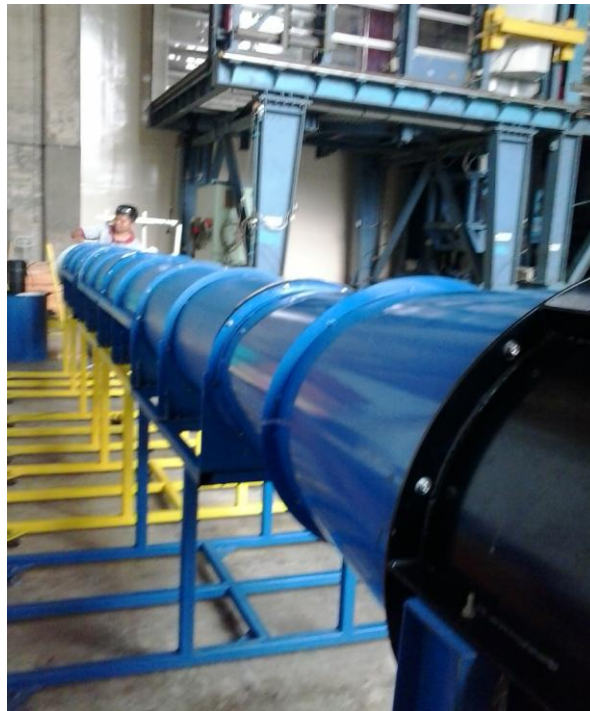
Fig. 2. Ducting Inlet, Open Outlet Fan performance testing facility
