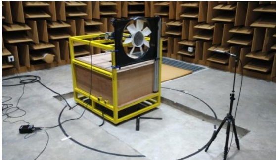
Fig. 3. Fan noise measurement in semi-anechoic chamber BBTA3.
