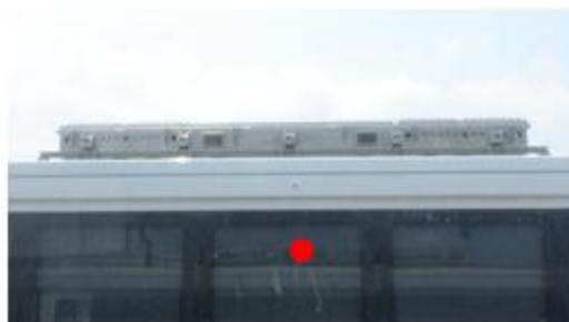
Figure 3: Microphone position for static measurement (outside view)
