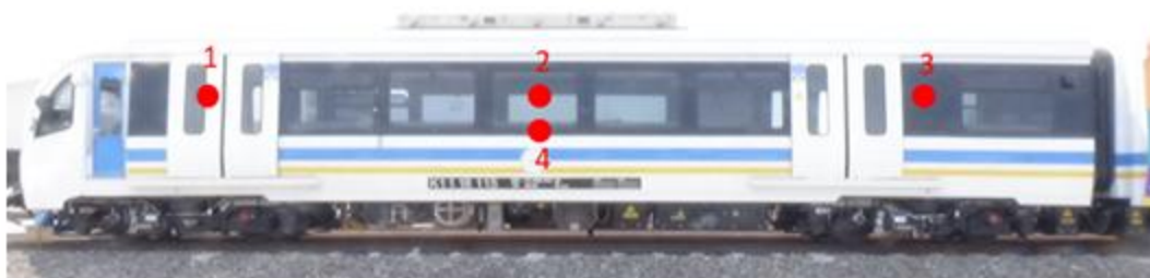
Figure 5 : Microphone position for dynamic measurement (outside view)
