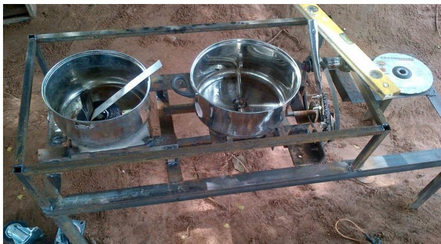
Plate 1. Fabrication process of yam pounding machine
