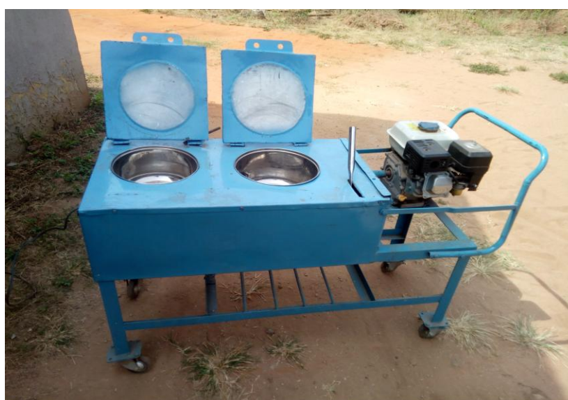
Plate 2a. Developed Yam Pounding Machine with Cooking and Pounding Chambers Open
