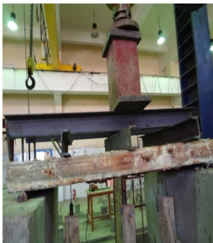
Figure (4). Schematic of flexure test setup.
