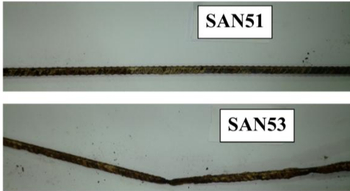
Figure (9). Photos for reinforcing steel bar after conducting the flexure test for slabs SAN51 and SAN53.
