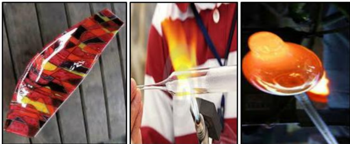
Figure 5: Process of Fusing or Vitrofusion, Process of blowing in torch with blowtorch and Process of blowing in cane [10].
