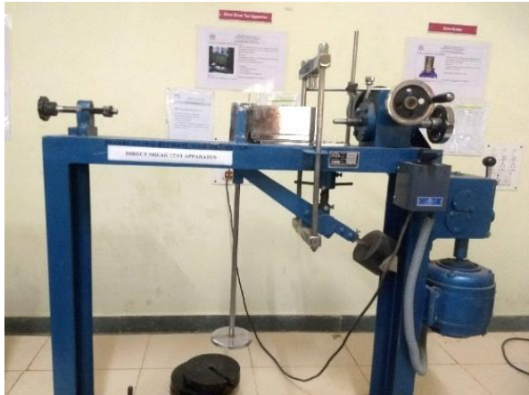
Fig. 3.4 Instrument setup for direct shear test
