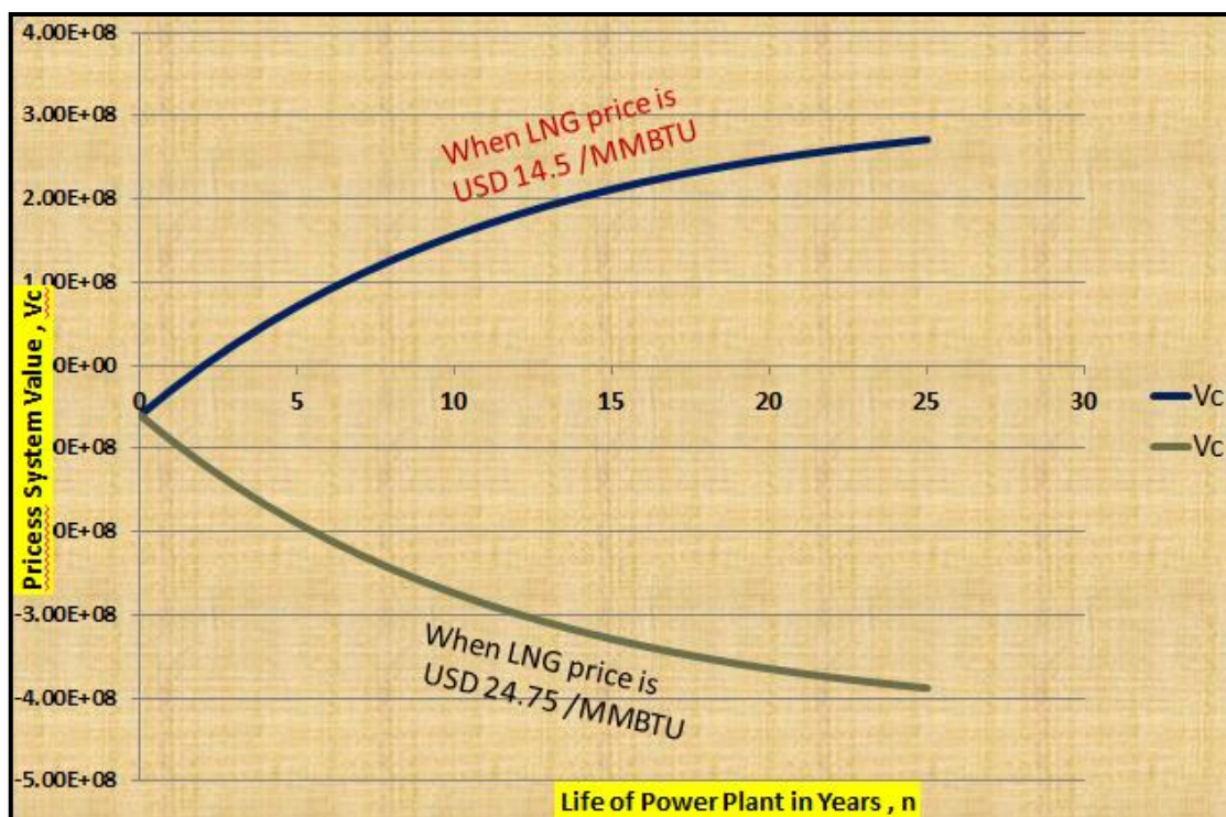
Fig 12 : Combined Plot of Process System Value ,”Vc” vs Life of Power Plant in Years,”n” (Case 1: LNG price = USD 14.5 per MMBTU as on August 2013) (Case 2 : LNG price = USD 24.75 per MMBTU as on April 2014)
