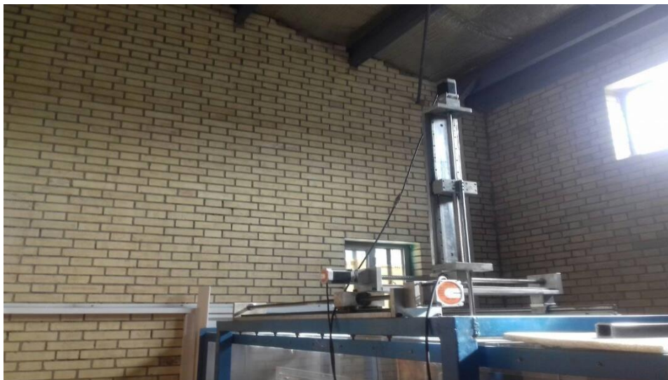
Figure 5: Probe Traverse System
