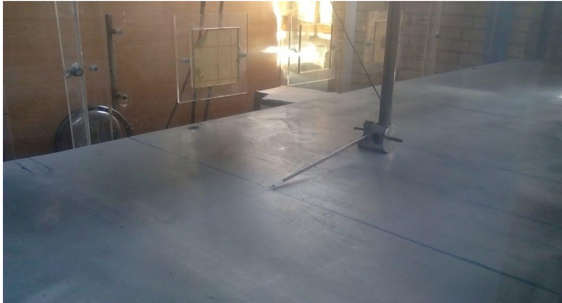
Figure 4: Hot-Wire probe while measuring the streamwise velocity on the flat plate in the test section
