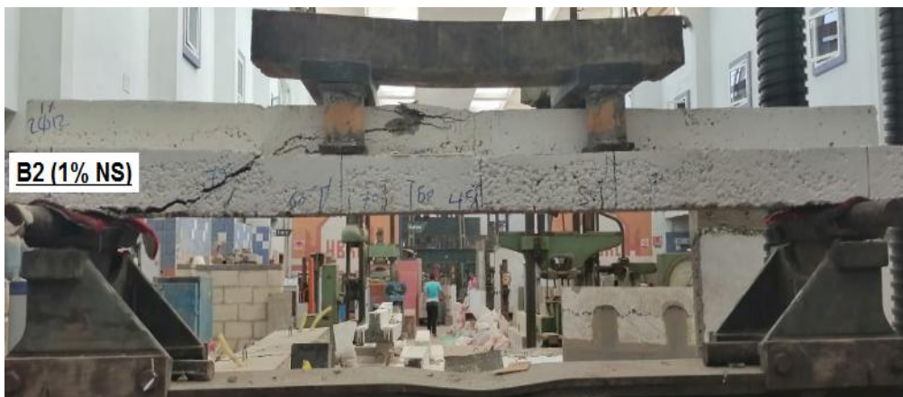
Figure (9): Crack pattern for control beam (B2)
