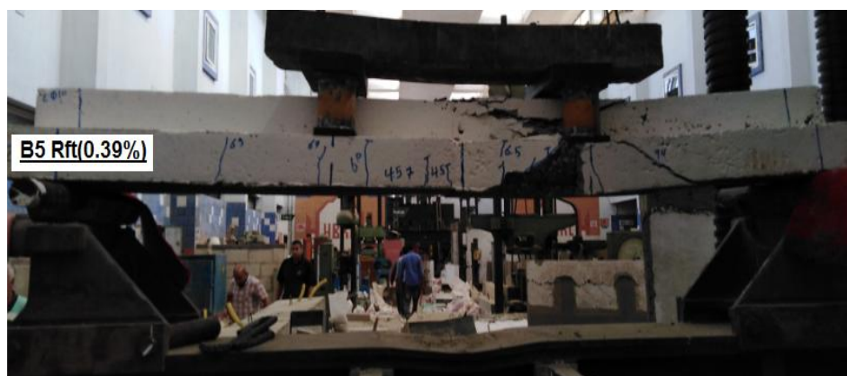
Figure (12): Crack pattern for control beam (B5)
