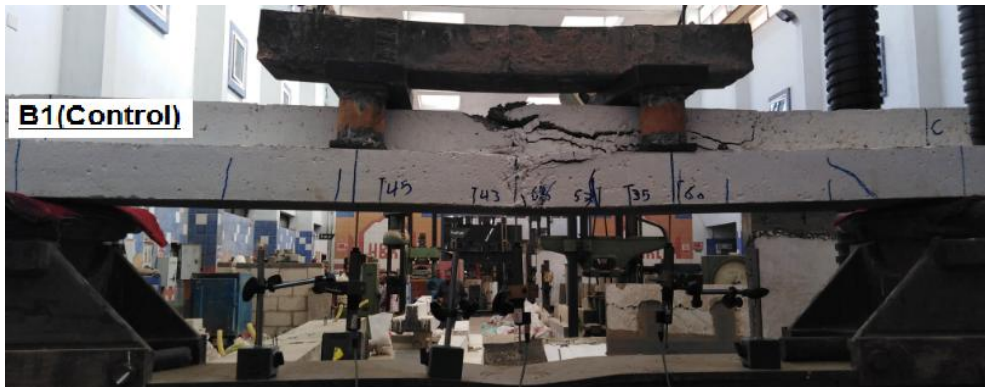
Figure (8): Crack pattern for control beam (B1)
