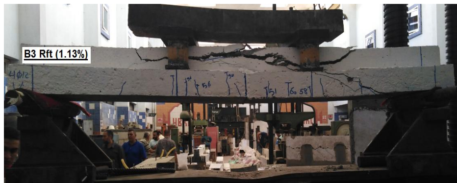
Figure (10): Crack pattern for control beam (B3)
