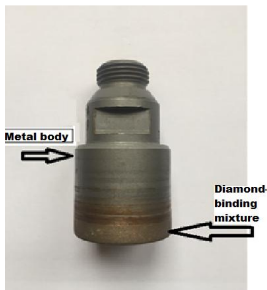
Figure 2 Drill used for glass drilling
