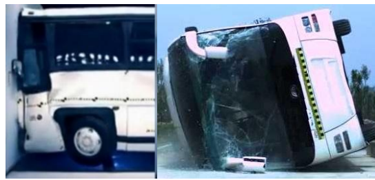
Figure (1): Bus frontal collision with a fixed barrier and Rollover accidents.
