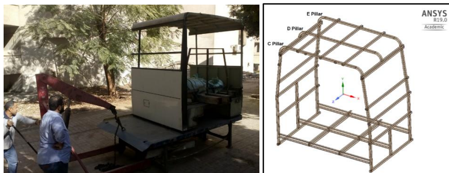
Figure (13): Bus Section Geometry and actual section on Tilt-table During Rollover Test.
