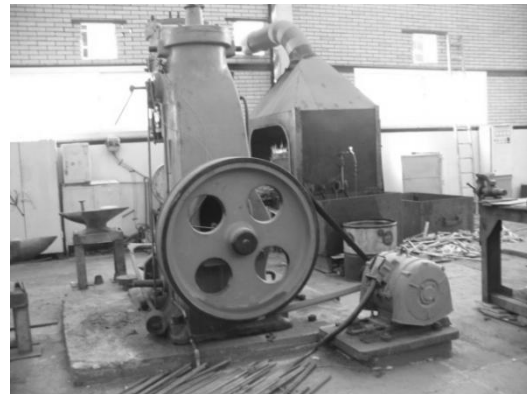
Fig. 7 Hammer with 100 kg. (220.46 lb.) dropping parts
