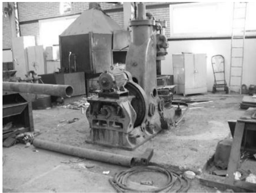
Fig. 6 Hammer with 250 kg. (551.16 lb.) dropping parts
