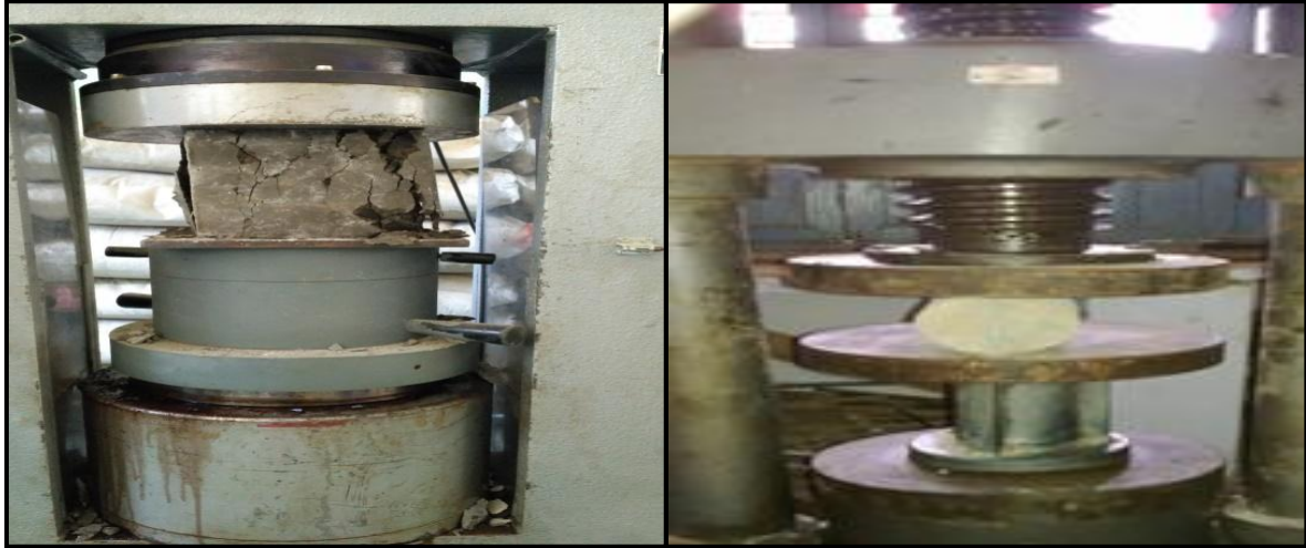
Fig 5.Compressive strength of cube.Fig 6.Setup for split tensile strength test
