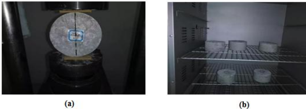
Figure 4: (a) Setup for pre-loading of specimens; (b) Setup for oven-drying of specimens
