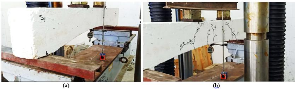
Fig. (14). Cracks Pattern for the Beam (BC 1)
