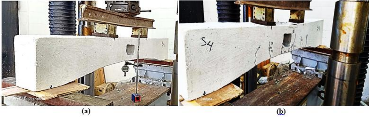
Fig. (16).Cracks Pattern for Beam (BFO 1)
