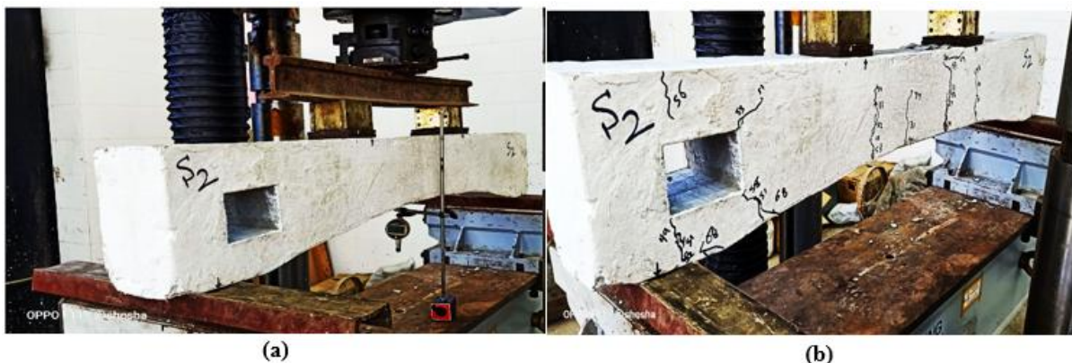
Fig. (15) Cracks Pattern for the Beam (BSO 1-1)
