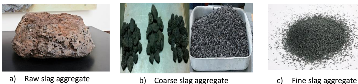
Fig.1 Blast furnace steel slag
