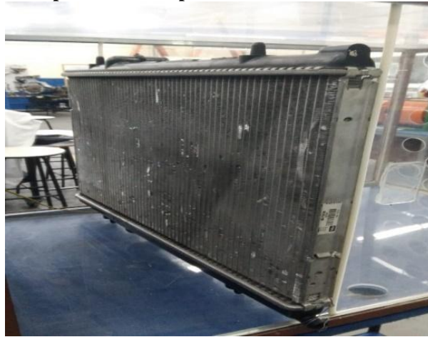
Figure 1- Compact flat finned tube heat exchanger (Automotive radiator)
