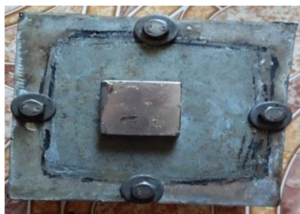
Figure 4: Curing of MRE under magnetic field.
