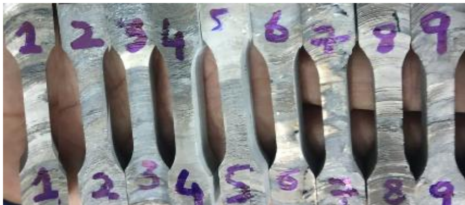
Figure 6. Tensile specimens as per ASTM E8/E8M-11.
