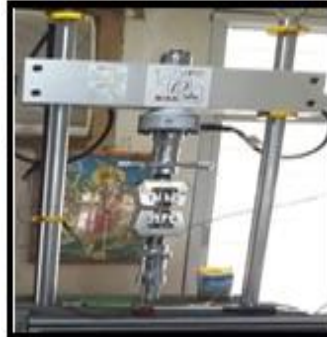
Figure 5. Nano plug and play servo-hydraulic tensile testing machine
