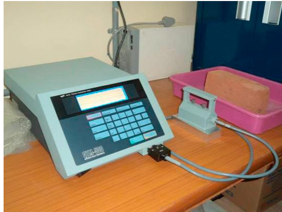
Figure 3: Contact hot-wire device (Quick Thermal Conductivity Meter: QTM-500) for measuring thermal conductivity.
