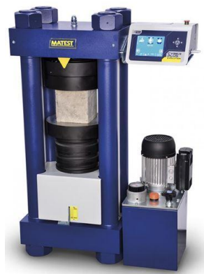
Figure 4: Concrete compression machine, 3000 kN, for measuring compressive strength.
