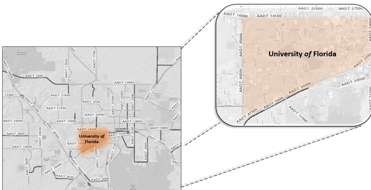
Figure 2: Average Annual Daily Traffic (AADT) 1 , the city of Gainesville and University of Florida.
