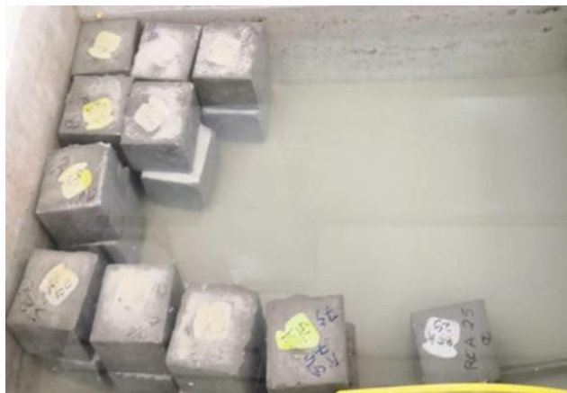
Fig 2: Curing Tank for the cube specimens
