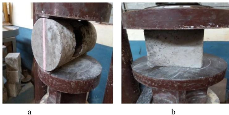
Fig 2a and 2b- Compression and split tensile test on cubes and cylinders.
