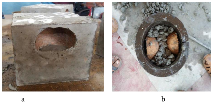
Fig 1a and 1b- Casting of cube and cylinder with coconut as filler.
