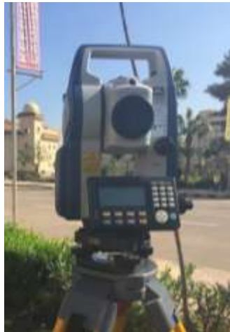
Figure 10: SOKKIA CX105 total station
