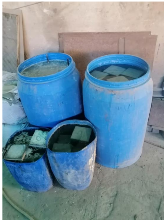
Figure 4. The curing of specimens
