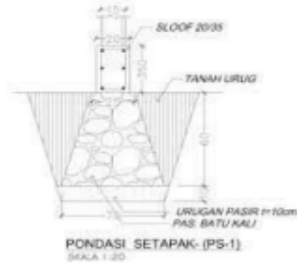
Figure 2.2 River Stone Foundation
