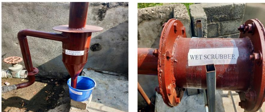
Figure 5. fabricated cyclone separator and wet scrubber for the experimental setup
