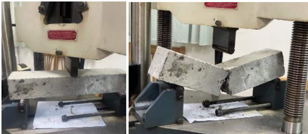
Fig. 12. Universal machine(300KN): (a) Beam during the test, and (b) beam after failure
