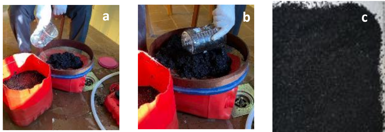
Fig. 3. Treatment of rubber tyre: (a), (b) Rubber tyre soaked in NaOH solution, and (c) Rubber tyre air dry
