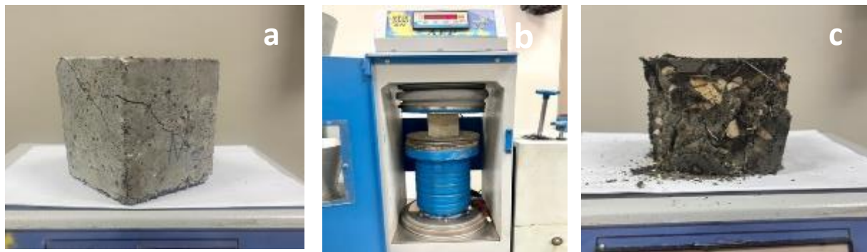
Fig. 8. Compressive strength machine: (a) M3 after the compressive strength test, (b) Cubic during the test, and (c) M7 after the compressive strength test.
