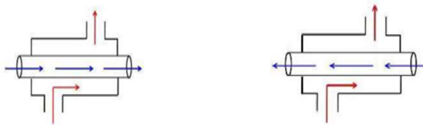
a. Parallel flow heat exchanger
