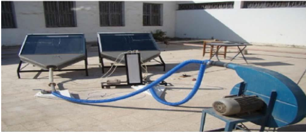
Fig. 8. Test-rig of finned heater and conventional heater [13].
