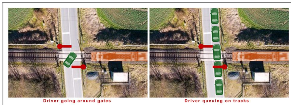
Figure no 1: Indicative examples of improper driving behavior that can contribute to crashes at at-grade rail crossings.
