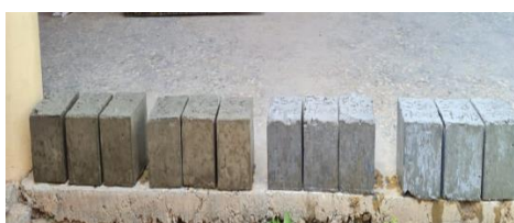
Figure 1: Hardened concrete specimens showing FF, FS, SF and SS
