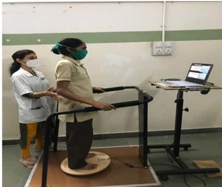
Fig. 1 wooden wobble board connected with laptop having software
